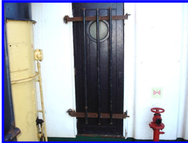
Extra strengthening on at risk doors mainly used in the construction of a secure room or citadel
